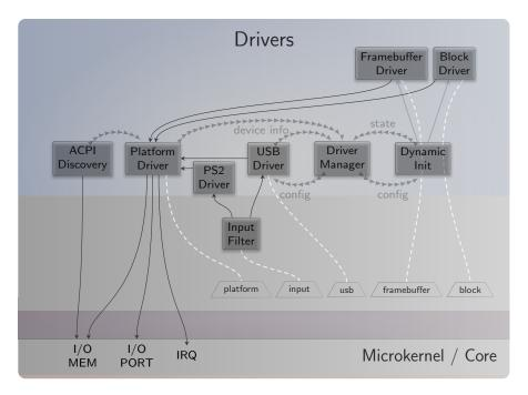
Figure 15: Services provided by the drivers subsystem
