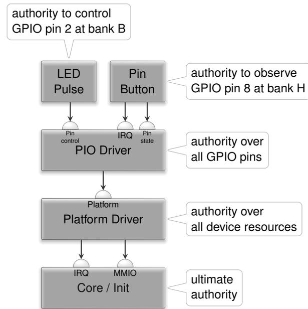
The higher up we get, the less influential the components become. Whereas the kernel has ultimate authority over everything, the reach of the pin-pulse component is limited to the control of the output signal of a single GPIO pin only.
