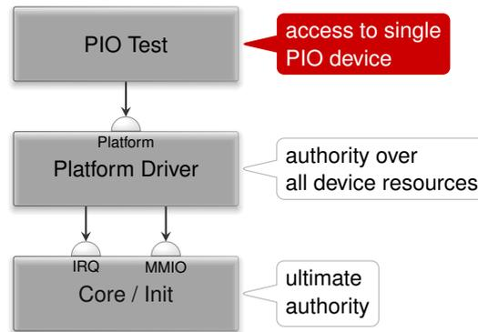
To integrate the notion the platform driver into our existing scenario of accessing general-purpose I/O pins via a to-be-developed PIO device driver, it is best to first sketch a run script that mirrors the picture above. We have to find a suitable name and location within our source tree for our designated driver component.
