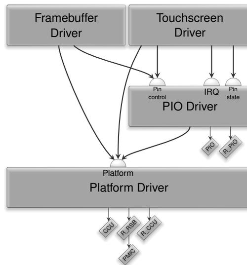
The framebuffer and touchscreen drivers no longer access the low-level system-control registers directly. Instead, the platform driver controls the reset, clock, and power states depending on the presence of its clients. Analogously, the driver's direct GPIO access of the direct pin-MUX manipulation is replaced by the use of the services provided by the PIO driver component.
