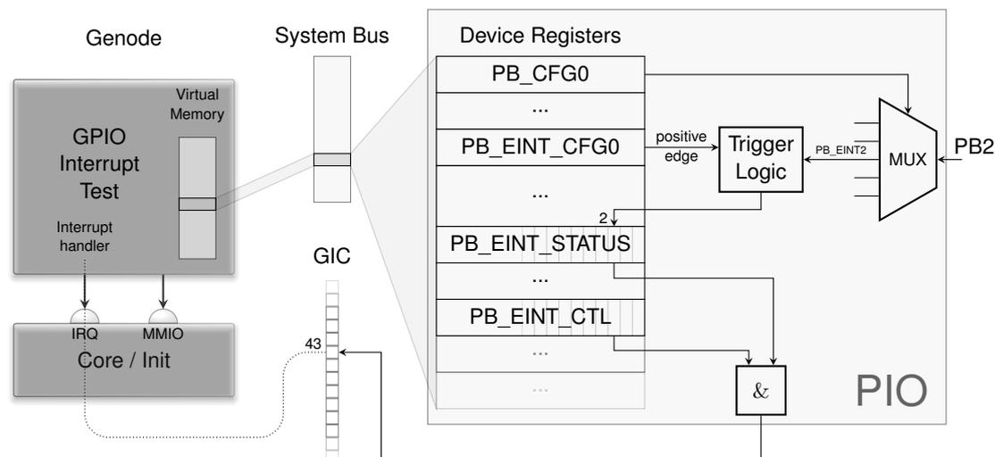
The exact conditions for triggering an interrupt can be configured for the pin using the PB External Interrupt Configure Register 0 (PB\_EINT\_CFG0). By default, the status goes to 1 as soon as a rising edge is detected. The other alternatives are falling edge, level-high (interrupt stays pending as long as the signal is high), level-low, and double edge (interrupt on any change of the signal).
