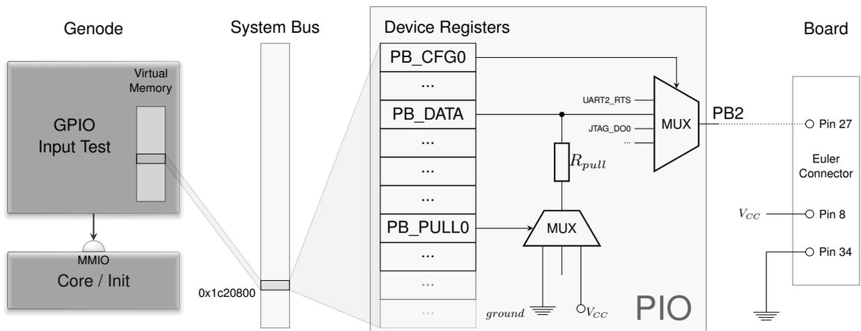
The pin 27 of the Euler connector goes to the PB2 pin of the SoC. Via the PB\_CFG0 register, we configure this pin to be used as general-purpose I/O pin reflected by bit 2 in the PB\_DATA register. The register set of the PIO device unit is visible at physical address 0x1c20800 at the system bus. Thanks to the MMIO service of Genode's core, our test component becomes able to access this register range as part of its virtual address space. So what's this PB\_PULL0 register shown in the picture?
